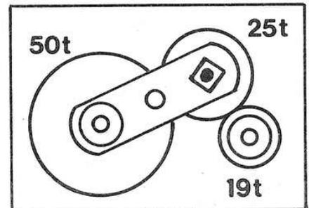
"This device can replace the free wheel made up of Pawls and Ratchet Wheel in some clocks, etc.," says Mr. Hauton.
