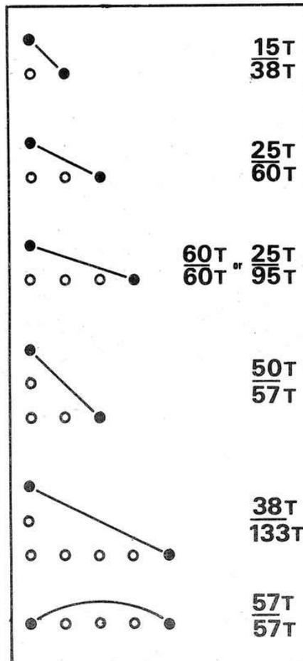
In addition to the above, Mr. Hauton says that, "For some difficult ratios, the unorthodox may be permissible, e.g. linking a Gear Wheel with a Sprocket Wheel via Sprocket Chain (Sprockets provide the factors 7 or 9 in compact arrangements)." He further goes on to say that in some arrangements, "A floating Pinion
