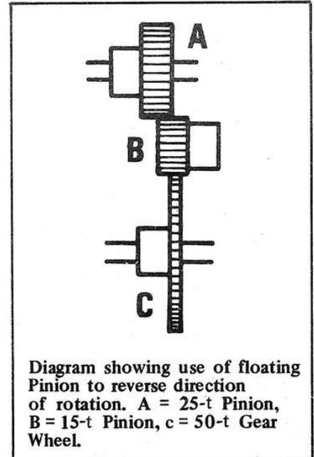
"The 19-teeth Pinion can be locked in the slotted hole of a Crank with a ¾" Bolt and two Nuts, the boss of the Crank being bolted to the frame of the supporting structure. Occasionally, a Gear is required to rotate free in one direction, and to do this a floating Pinion is pivoted on the Crank, but the Crank boss is loosely journaled on the shaft taking one of the Gears, thus:
