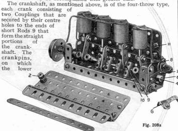
ends of the connecting rods 8 are mounted, each consist of a 1" Screwed Rod that is secured by lock-nuts 10 in the transverse end tapped holes of each pair of Couplings, the upper extremities of the connecting rods being carried on Setscrews inserted in Collars on the ends of the piston rods. The complete crankshaft is journalled in 1½" Strips 4, and care should be taken to see that all Grub Screws and lock-nuts are tightened very securely in order to prevent the possibility of the crankshaft
