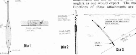
facilitate float-changing and to enable a float to swing freely on the line even though it is set at a fixed depth.
