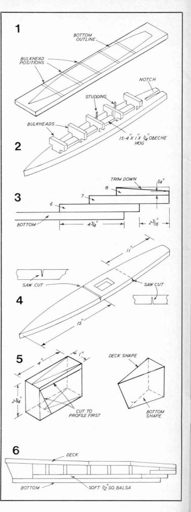
quite straightforward. Leave to set and then trim off the top of part 8 at an angle so that its depth at the rear end is reduced to 4 in. (You can, if you prefer, do this trimming before cementing part 8 in place.)
