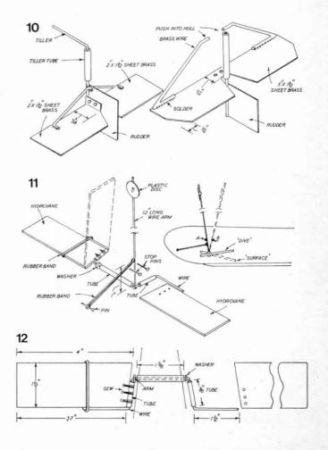
material, pierced to mount on the wire but free enough to be slid up and down. This wire is kinked about 1 in. up from its pivot point and a rubber band is taken from this kink and fastened to the hull side with a pin. A further pin 'A' is then pushed into the hull side to act as a forward stop, limiting the 'dive' position assumed by the hydrovanes. This pin position, and the position of the pin anchoring the rubber band which controls the band tension can only be determined by experiment.
