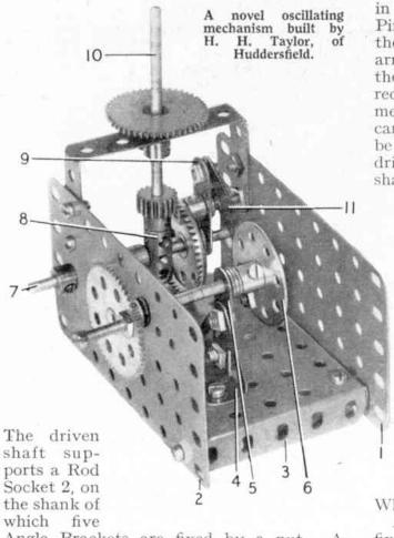
Angle Brackets are fixed by a nut. A Threaded Pin is held by its nut in each Angle Bracket, to make a star wheel with
