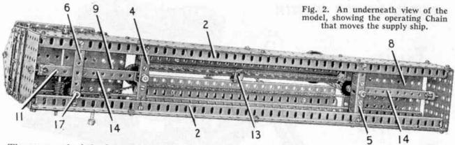
The rear end of the boat-house is filled in by two 3" and two  $3\frac{1}{2}$ " Strips, two  $2\frac{1}{2}'' \times 1\frac{1}{2}''$  Flexible Plates and a  $2\frac{1}{2}$ "  $\times 2\frac{1}{2}$ " Triangular Flexible Plate. These are bolted together and attached to Angle Brackets fixed to the sides. The boat-house roof is a Hinged Flat Plate supported by Obtuse Angle Brackets. At the front a second 2½"×2½" Triangular Flexible Plate is attached to Angle Brackets.
