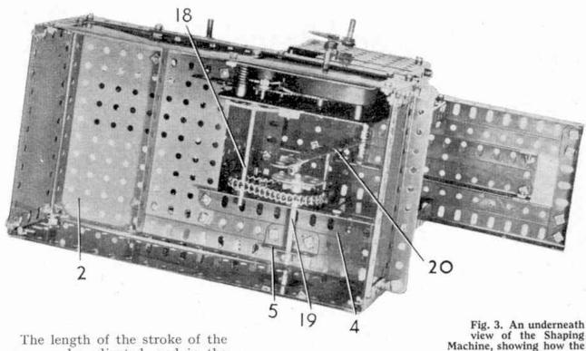
The length of the stroke of the ram can be adjusted, and in the larger machines a "quick return" motion is provided, the tool being run back to the starting point of its travel, ready for a new cut, at a higher speed than when cutting. This saves much valuable time.
