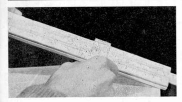
Here's a precision instrument you can make for a shilling or less, using balsawood and the printed scales reproduced alongside. And construction time is only a matter of an hour or so!
