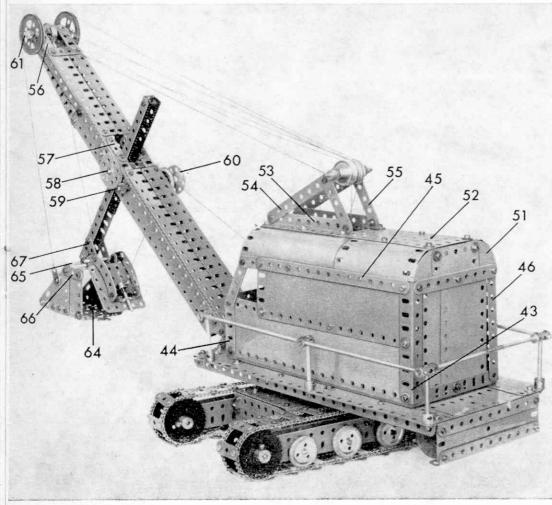
tion on the upper side. An Angle Girder 20 is attached to a 5½ in. by 1½ in. Flexible Plate and is bolted to the rear of the base. To balance the weight of the jib a piece of lead or a length of steel shaft is tied to Angle Girder 21.
