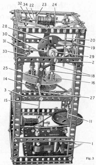
Keyway. The Rod with Keyway is fixed in place at one end of the framework and the uncovered wire is led along its slot so that it passes through the centre of the thread carrying assembly. Thus this assembly is able to rotate on the 4" Rod with Keyway without twisting the wire, and the wire can be drawn through the centre of the thread carrier. The uncovered wire is drawn from a reel mounted at one end of the frame.
