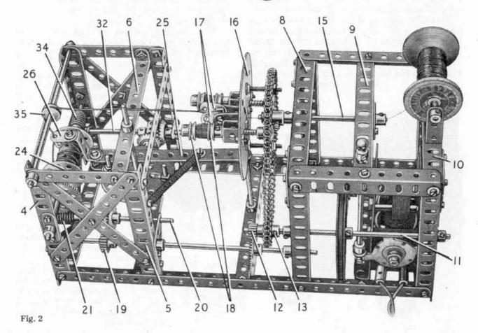
Fig. 1. An attractive model of a Wire Covering Machine designed for covering wire with two layers of cotton or other insulating material.
