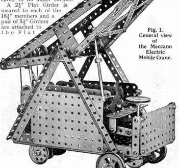
Girders and also to the end holes of the  $18\frac{1}{2}''$  Girders. A pair of  $13\frac{1}{2}''$  compound girders, each built up from one  $5\frac{1}{2}''$  and one  $9\frac{1}{2}''$  Girder, are also bolted to the Flat Girders, while their upper ends are secured to the front of the jib-frame.
