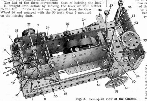
with crane jib removed.
