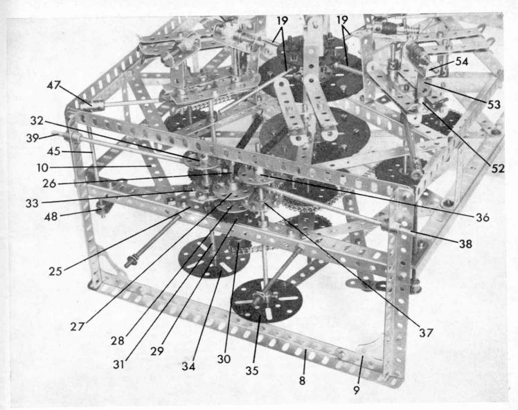
12½ in. Angle Girders. This Rod carries, between the Angle Girders, a Collar, two eight-hole Bush Wheels 27 and 28 and a 1½ in. Sprocket Wheel 29, this Sprocket Wheel and the Collar holding the Rod in place. Bush Wheels 27 and 28 each carry four Bolts, in adjacent holes, held in place by Nuts. It is advisable, incidentally, to secure the Bush Wheels on the Rod with two Grub Screws in each boss. A ¼ in. Sprocket Wheel 30 is added to the lower end of the Rod.
