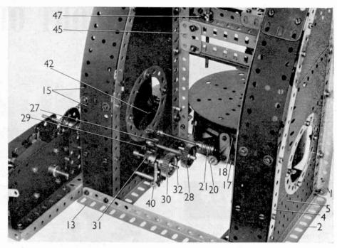
supports a  $2\frac{1}{2}$ " Rod 58 carrying a  $\frac{7}{8}$ " Bevel Wheel that engages with the  $\frac{7}{8}$ " Bevel Wheel mounted with a Key Bolt 59 on the Rod with Keyway 55. The tool chuck is a short Coupling fixed in the lower end of Rod 58.
